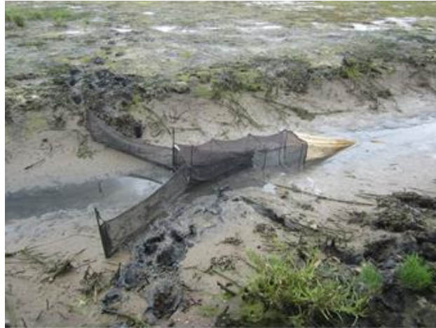
Plate 3 Small winged fyke net with 1mm cod-end and 3mm micromesh panels and wings.
